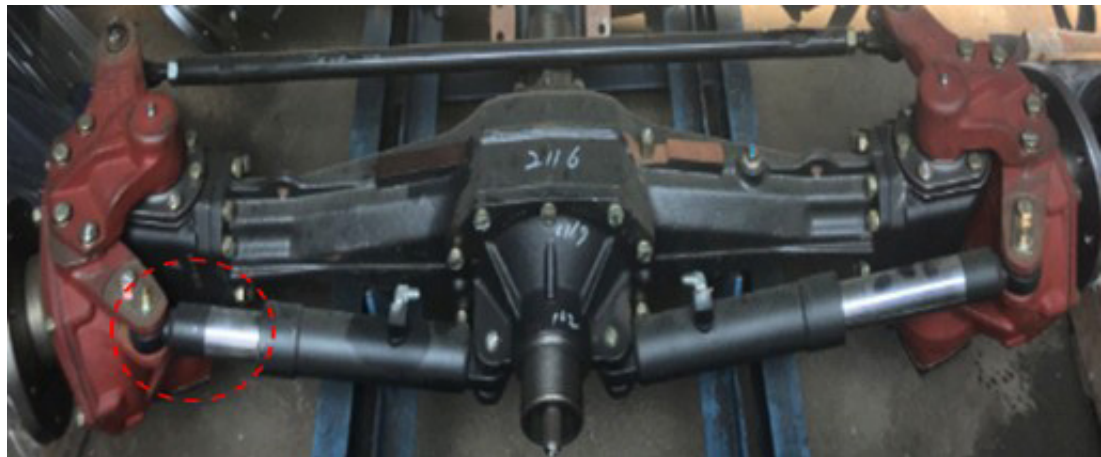
Fig. 4. Sensor installed on the front axle of the harvester
