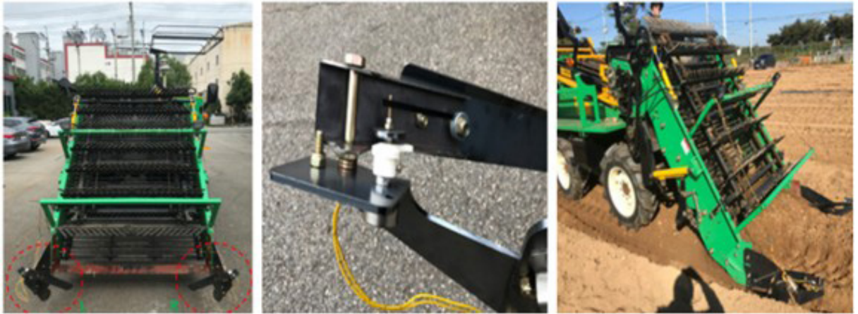
Fig. 3. Ridge detection sensor method and performance test on the ridge line
