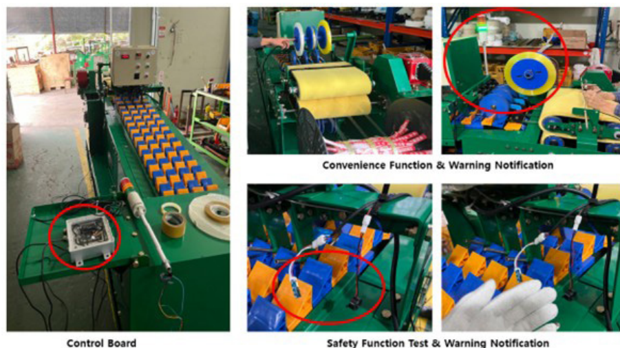
Fig. 2. Early model of smart multi-functional notification system for sweet potato shoot attachment device
