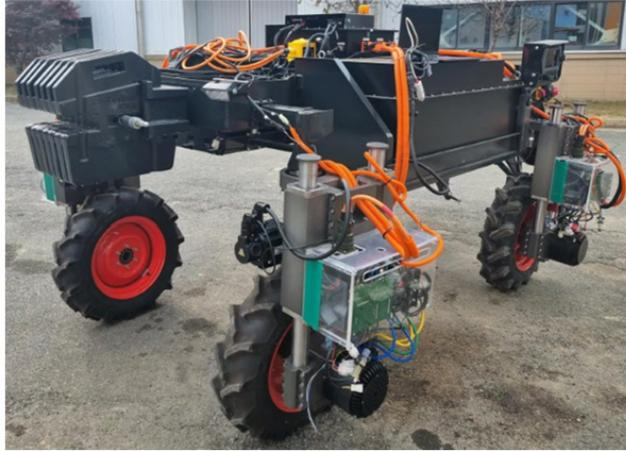
**Fig. 1.** Four-wheeled electric drive field agricultural platform
