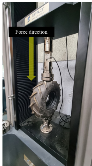
Fig. 4. Measurement of tire vertical stiffness using universal material tester and jigs (Park et al., 2024, p. 320).
