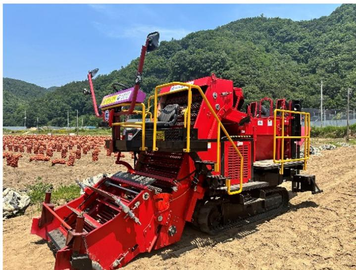
**Fig. 1.** A photo of self-propelled underground crop harvester used in this study
