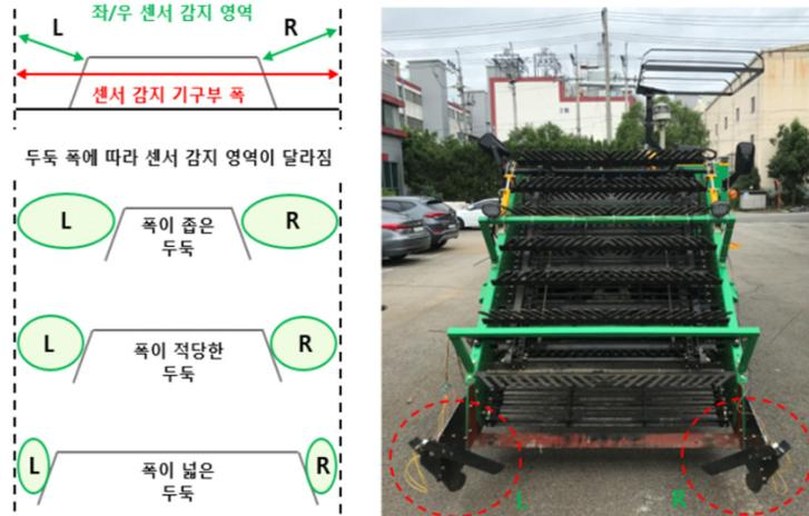
**Fig. 4.** Ridge detection principle and ridge detection sensor mechanism
