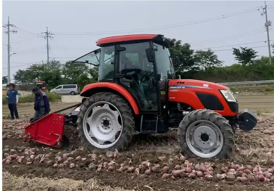
**Fig. 2.** Field experiment of each digging-type onion harvesters
